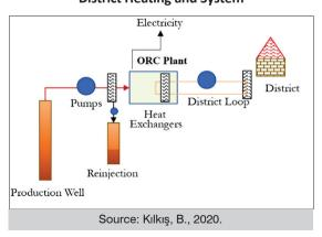
Figure 15. Utilizing Waste Heat from ORC for District Heating and System
