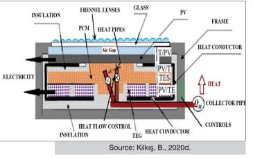
Figure 13. Advanced Photo-Voltaic-Heat Systems with high Efficiency
