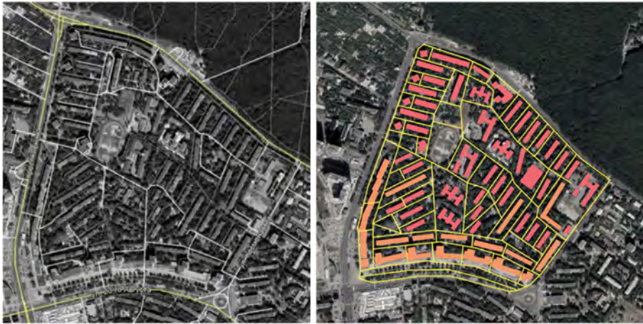
Figure 5: structural diagram (right) with long housing blocks (orange), short housing blocks (red), and existing transit network (yellow).
