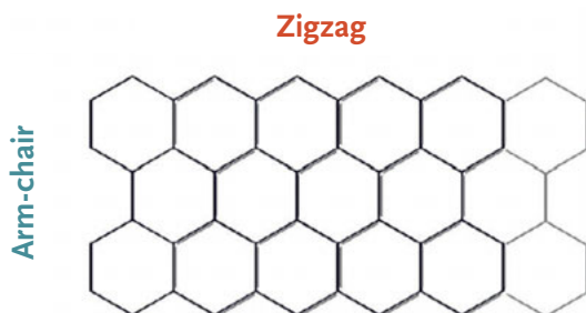
Fig. 4: 0 degree (armchair) or 30 degree (zigzag) fold edges.
