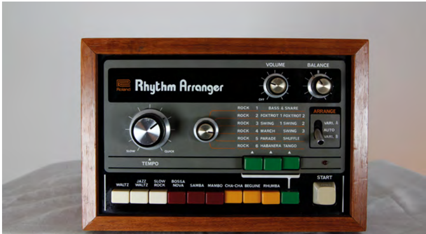
Figure 6: The Roland TR-66 Rhythm Arranger might be regarded as the last, pure preset drum machine produced by the renowned manufacturer Roland. It came in a handy shoebox size. The presets included possible combinations and the arrangement feature can clearly be seen in the figure. All subsequent models provided expanded options for programming and arrangement, until the drum machines of the 1980s brought about true liberation in groove creation via a programmable matrix. Photo: Robert Michler, 2022
