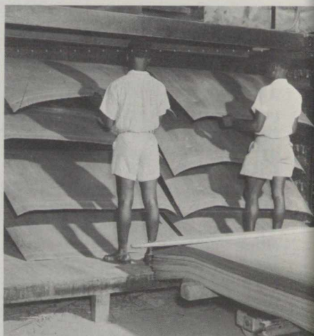
AT NEARBY LUKULA the sheets of corestock and veneer are glued together to form plywood. This factory is also owned by Agrifor and was built with the aid of U.S. Plywood. The plywood is finished and packaged for shipment to customers in the Congo, in Europe, and in the United States.
