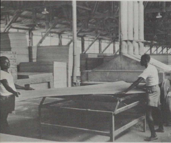
AT NEARBY LUKULA the sheets of corestock and veneer are glued together to form plywood. This factory is also owned by Agrifor and was built with the aid of U.S. Plywood. The plywood is finished and packaged for shipment to customers in the Congo, in Europe, and in the United States.
