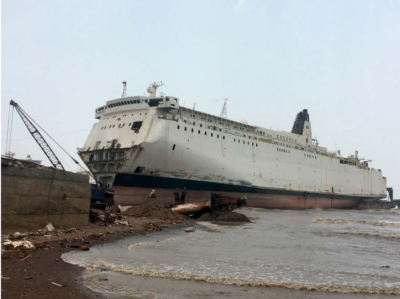
Figure 5. Shipbreaking in progress with a cut being made on the nose of the ship (Photo: Ayushi Dhawan).
