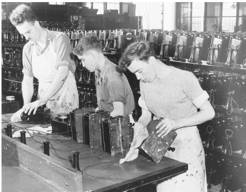
Figure 4. “These [wall sets] have been repaired and reconditioned and are being cleaned before being refinished. The Cleaners are left to right, John Wilkinson, Gordon Hann and James Dunn.” (Image and caption appeared in Blue Bell , Bell Canada’s employee magazine, Oct.1942, BCA, A-38716-04)
