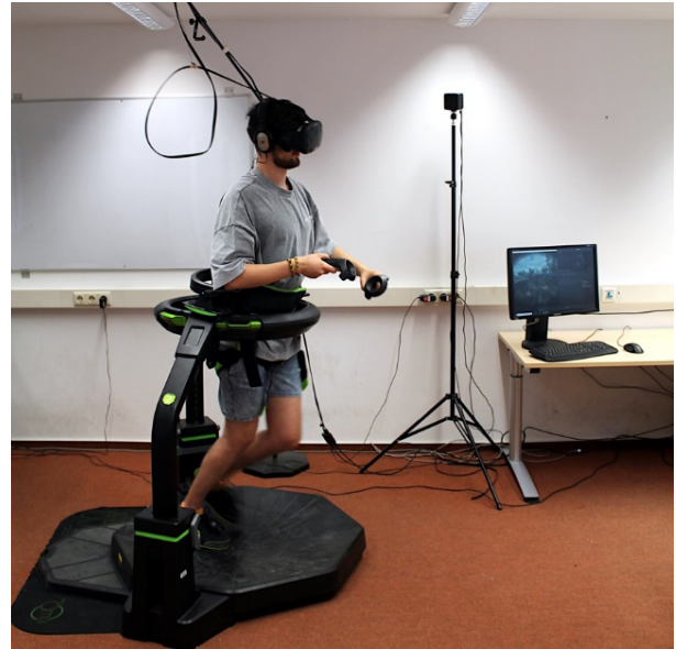
Figure 4. Laboratory setup of the Omni gaming experimental condition.
