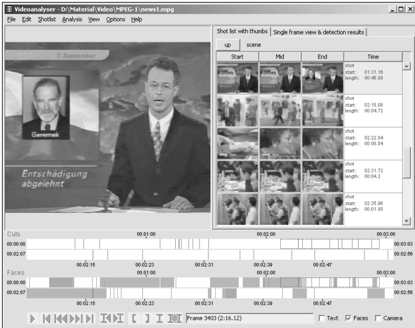
Figure 1: The main window of Videana . On the left side, there is a window for playing a video. There are two timelines at the bottom which visualize the analysis results for the temporal segmentation of the video into shots as well as for face detections. The vertical lines in the Cuts timeline represent cuts (abrupt shot changes), the colored (here: grayish) areas in the timeline Faces mark the sequences where a frontal face appears. Two timelines are presented for each kind of event: the upper one represents the total duration of a video, whereas the lower one zooms into a certain time period which can be selected in the upper timeline and is surrounded by a rectangle. Further timelines are displayed in case that the corresponding analysis results or user annotations are available for the related events of camera motion, superimposed text or audio events. On the right side, the temporal segmentation is presented in another way. Single shots are represented by three frames (beginning, middle, and end frame of a shot). By a mouse click on an icon, the related video frame is accessible directly, while a double click starts playing the video from this position.
