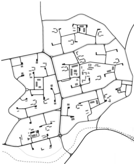
Figure 3.5: Fragment of the plan of the Ruashi neighborhood, indicating the public facilities and the main road infrastructure with the characteristic dead end streets. Source: scheme drawn by Céline Fenaux, based on archival material, 2010.
