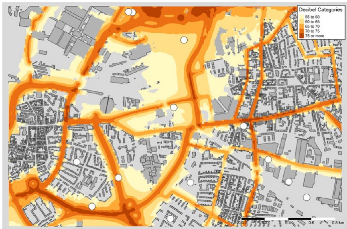
Figure 1 Map section of the city of Cologne with road traffic noise at its corresponding day, evening, and night mean decibel values and fictional respondents' geo-coordinates (data sources: OpenStreetMap Contributors 2017 and German Environmental Agency/EIONET Central Data Repository 2016).
