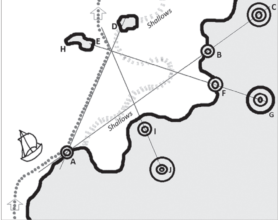
Fig. 53 Sketch on the use of transit lines, based on a rather similar situation in reality. Close to the coast are shallows, but it is well known that they extend to the islet D and further out. To avoid those the skipper goes in line with A-B-C at first, but at A he turns to port in order to go towards D, but, as he already knows, not too close to D. To know where to turn next time he fixes his gaze towards I-J and F-G. He then could sail quite close to the steep island H. The points given letters are all named in the formula of the transit lines and represent an important part of the place name flora in the maritime landscape. (Drawing: Christer Westerdahl & Erik Hoops)
