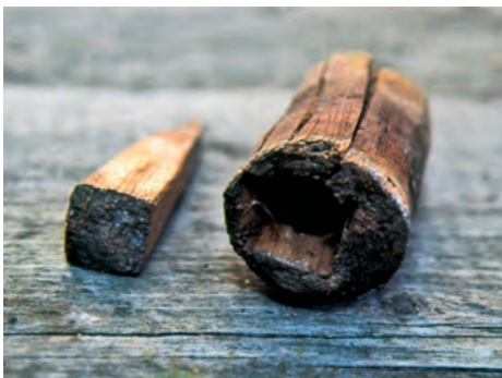
Fig. 44 Dowel and its wedge from a wreck of a ship built on the river Ångermanälven, probably a haxe , a local river barge type of the eighteenth century. (Photo: Christer Westerdahl, 1984)
