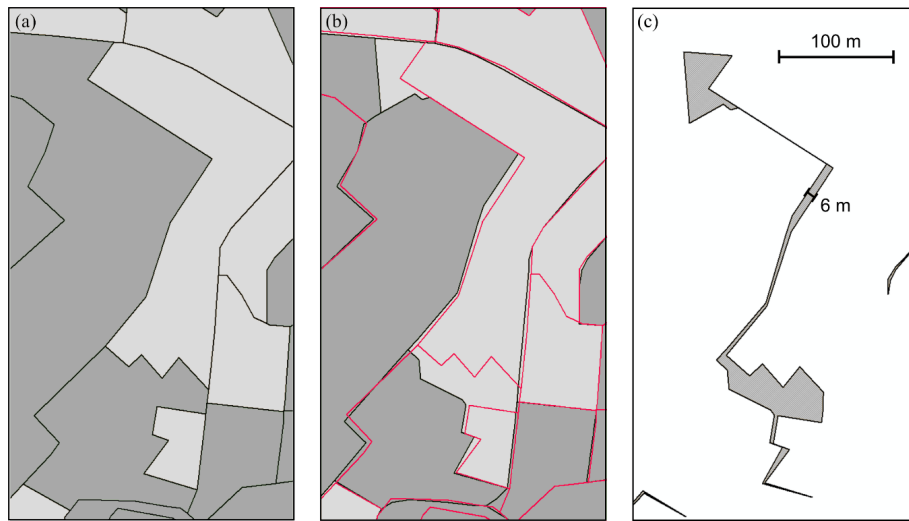
Figure 5. Small position changes of different land use polygons: (a) land use example Date 1; (b) land use example Date 2 (previous boundaries in red); (c) patch of detected land use changes with sliver polygons.
