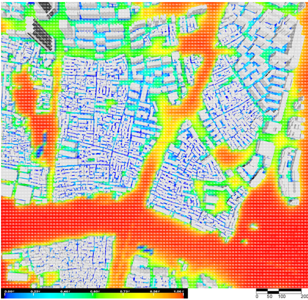
Figure 10. This figure shows Chengnan, an historical area of inner Nanjing, China, SVF calculated at 10m intervals.
