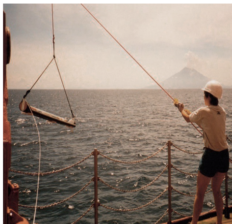
Figs. 19a–b. Preparations of RAFOS floats on deck of the POSEIDON and the SONNE. The transparent housing of the instrument consists of hardened borosilicate glass (left). The launch procedure (right) is achieved by a cradle with unsymmetrical buoyancy on its long side. After a predetermined time RAFOS floats release a ballast weight, return to the surface and upload their recorded data via satellite link to a ground station. Typically, their in-situ mission lasts between one and two years. (Photos: W. Zenk)
