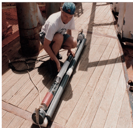
Figs. 19a–b. Preparations of RAFOS floats on deck of the POSEIDON and the SONNE. The transparent housing of the instrument consists of hardened borosilicate glass (left). The launch procedure (right) is achieved by a cradle with unsymmetrical buoyancy on its long side. After a predetermined time RAFOS floats release a ballast weight, return to the surface and upload their recorded data via satellite link to a ground station. Typically, their in-situ mission lasts between one and two years. (Photos: W. Zenk)
