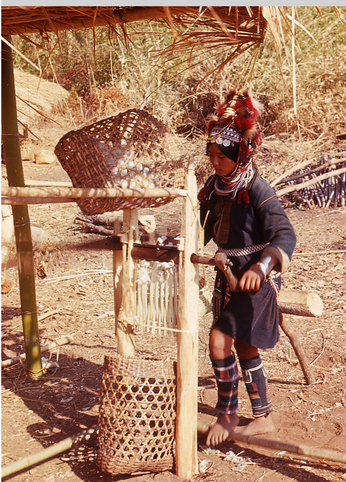
Seeding cotton: Cotton is put into the machine between two rollers which revolve in opposite directions. The cotton fibres are transported through these rollers and are thus separated from the seeds which had remained on them. Akha village, Chiang Rai Province 1965
