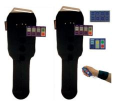
Figure 1: Sensor-wristband with multiple marker facility
