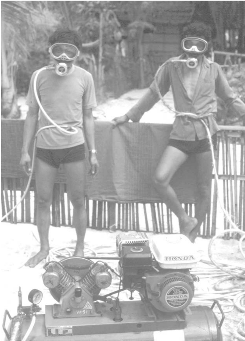
Fig. 3.4. Hookah equipment demonstrated by two Makassarese fishermen of South Sulawesi. The fishermen are connected by air hoses to the same air compressor.
