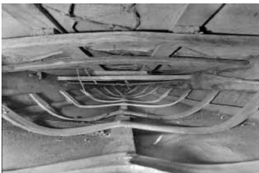
Fig 84. The kayak is very flat-bottomed and a glance inside the vessel for and aft shows clearly that most of the ribs in the frame have been pressed up, probably because it has lain directly on a flat floor for more than 30 years. On the drawing in fig. 83, the keel has, however, been straightened out in that the distance from the keel to the upwardly bowed ribs has been added from the bottom of the keel. It has a length of 5.9 m and is 60 cm at its broadest point. Two paddles accompanied the kayak, one lacking fittings whereas the other, which was made from very fine-grained dark driftwood, has both fittings and bone knobs. Photo by Werner Karrasch, Viking Ship Museum.
