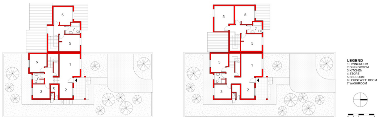
Figure 33. The Umudugudu Kigali 2020: Ground and first floor twin house types 2 and 1. Drawing by Manlio Michieletto.
