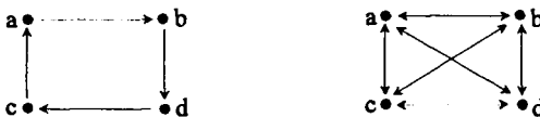
Figure 19.4. A cycle in an intransitive structure (left side) will be completed to a clique in a transitive structure (right side).
