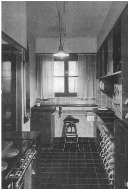
FIGURE 1 The Frankfurt kitchen, designed by Margarete Lihotzky, 1926. It is divided from the living room by the wall on the left. The jug-drawers (lower right), ready-labelled with the 'ideal' hygienic foodstuffs, proved particularly unpopular with housewives. The drawers named foods which they did not like, and did not have storage for potatoes.
