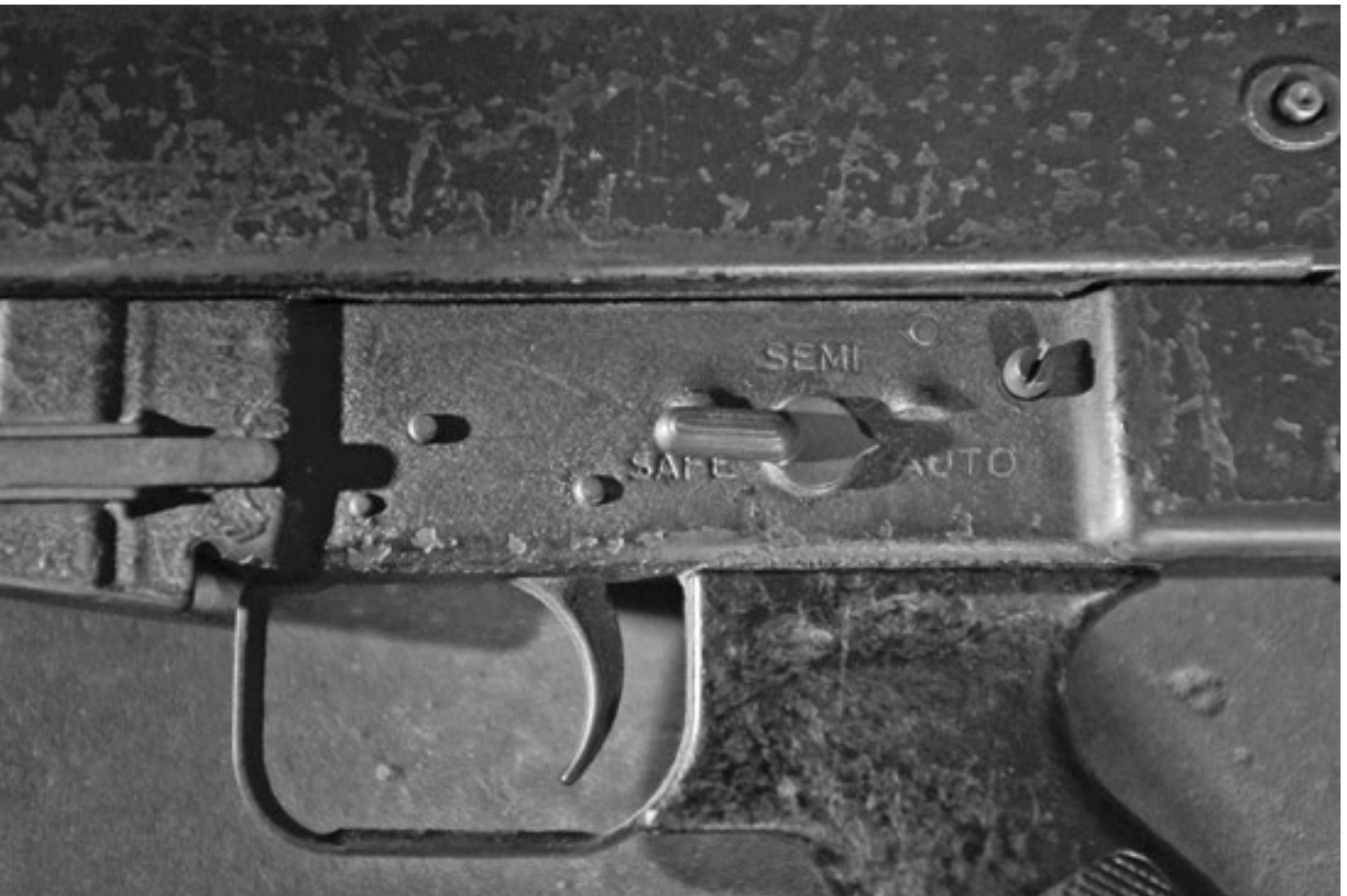
Safety mechanism on a US-American-manufactured Colt M16A1 5.56mm calibre assault rifle set to full auto-mode.
