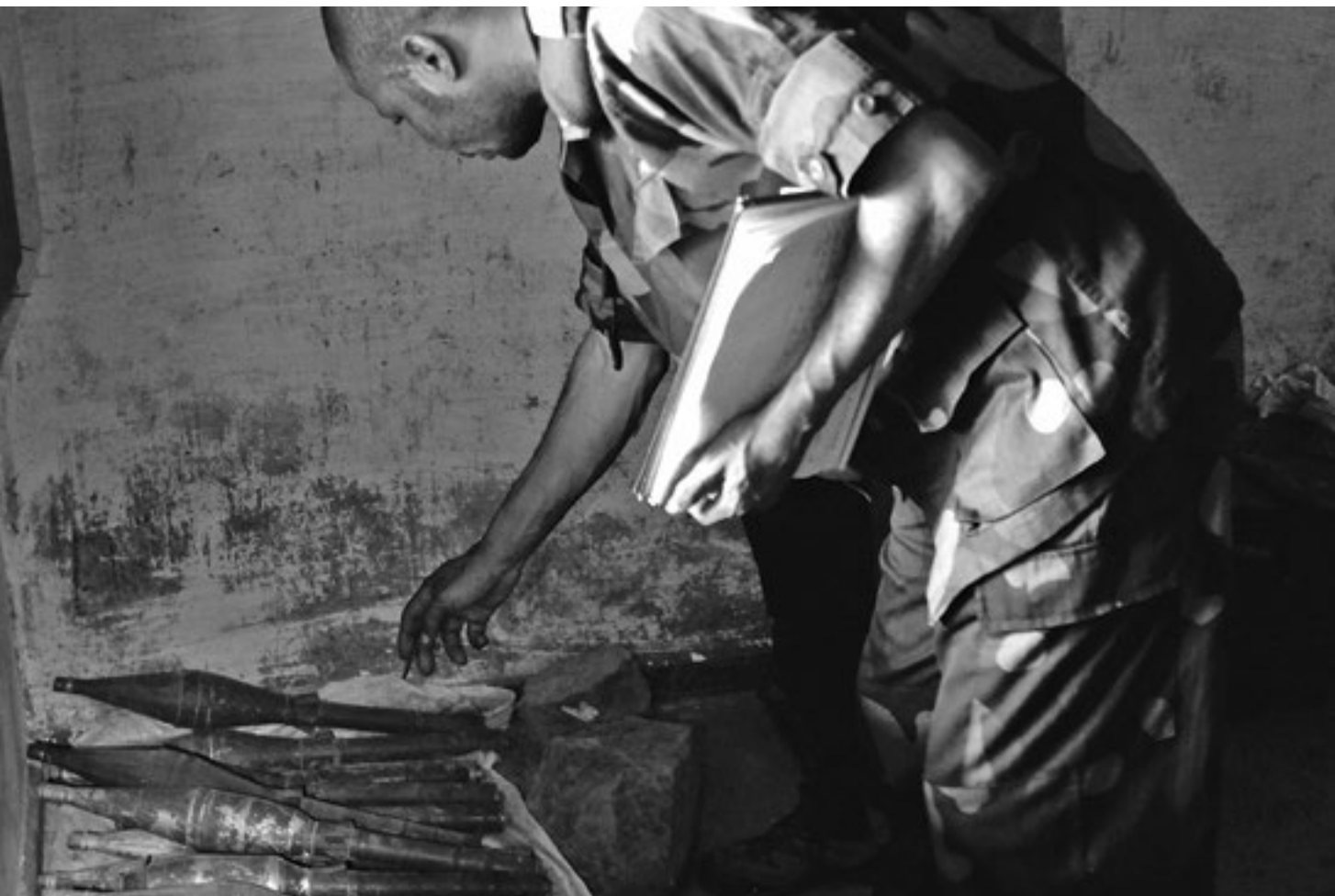
The assessment team examines a collection of RPG7 warheads, many of which are stored directly on the floor next to flammable phosphorous and not equipped with a security mechanism. Bokala munition depot, October 2015.
